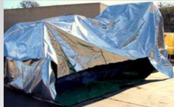
Unprotected metals begin to corrode immediately, so even JIT (just in time) manufactured parts will benefit from VCI protection.
